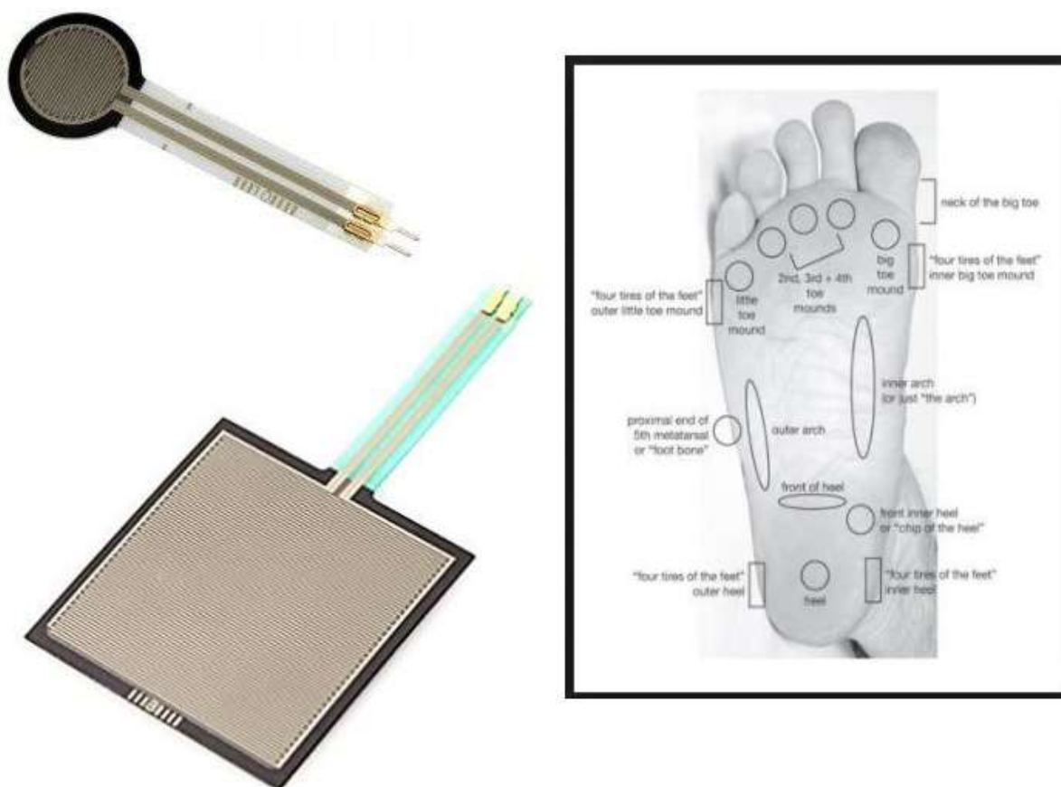
Figure 2 shows force sensors and potential pressure points for gait analysis
